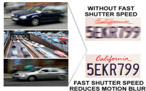
Figure 5. Motion blur reduction by fast shutter speed camera
